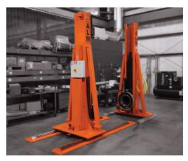
Fixed Headstock and Adjustable Tailstock
