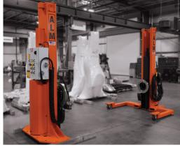
Fixed Headstock and Mobile Tailstock
