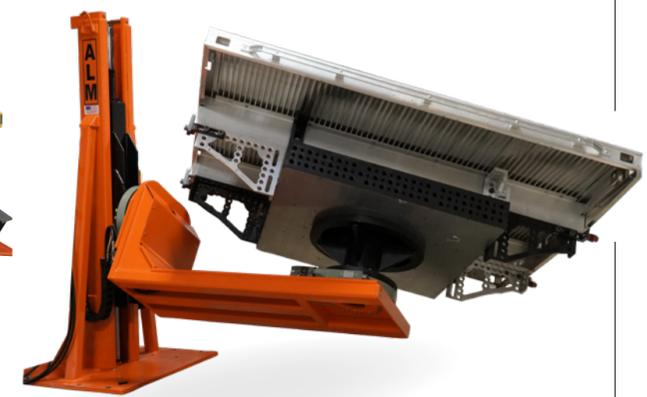
**Elevating Skyhook loading capacity:** 3,500-12,000 lbs.
