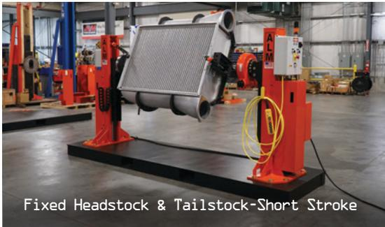
Fixed Headstock & Tailstock-Short Stroke
