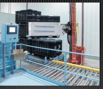
ALM lift moving a nested ProBox from supply conveyor and turning 90° to place it on the assembly conveyor.
