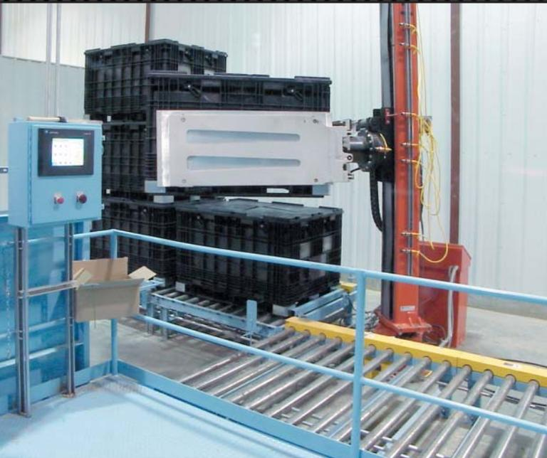
ALM lift moving a nested ProBox from supply conveyor and turning 90° to place it on the assembly conveyor.
