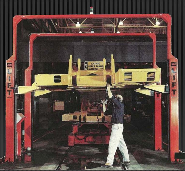
At this lift/load station on an assembly line, a four column, ALM Assembly Positioner holds a heavy component for work beneath it.
