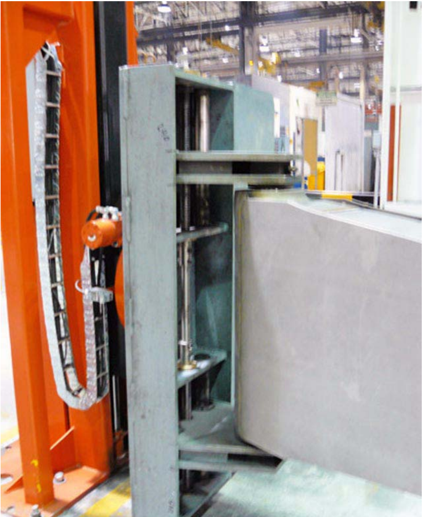
Fixed Headstock Adjustable Tailstock – 25,000 LB Capacity – 92” Vertical Travel
